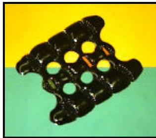
Figure 2 - Ferrofluid pattern created by an array of three "ringed" cow magnets.
