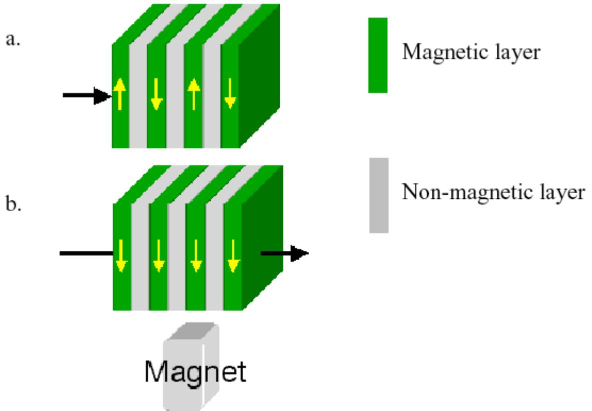
Figure 1: GMR materials are made from alternating layers of magnetic and non-magnetic metals that are nanometers in thickness.
