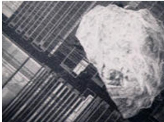
**Figure 11.** This enlarged image of a grain of salt on a piece of a microprocessor illustrates the small size and complexities of a microprocessor and the importance of clean rooms in manufacturing them.
