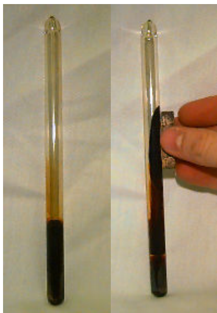
Figure 1 - Pulling ferrofluid up a tube with a strong magnet.
